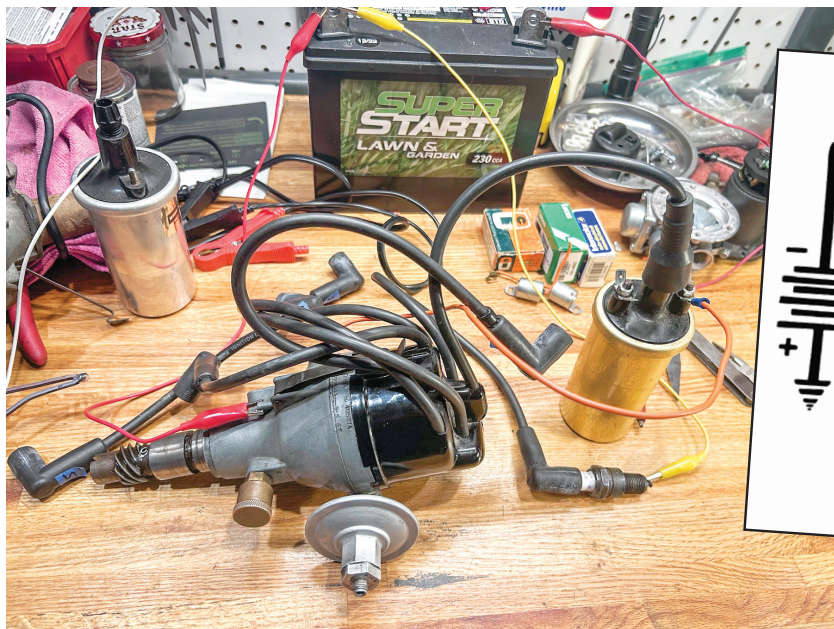
Coil and distributor bench test.
