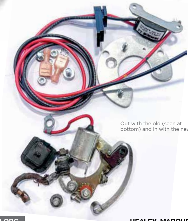
The original points, condenser and rotor. Keep the rotor!
